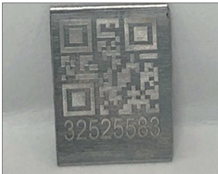
Figure 1: QR code and DNI number engraved by laser.
